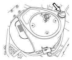
Now insert the dipstick again. The dipstick should be completely screwed down
